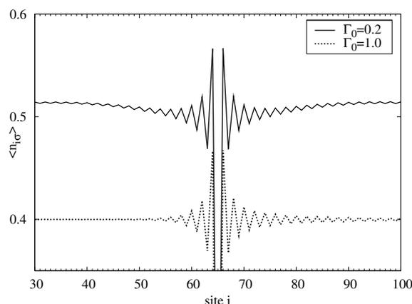
**Figure 3** Occupation of sites in the vicinity of the impurity for a 129-site nanowire. The temperatures of the electrodes are  $k_B T_L = 0.11t$  and  $k_B T_R = 0.01t$ . The values of the coupling constant are indicated in the legend. We have assumed the impurity potential  $U = 4t$  and the zero bias voltage. The curve for the  $\Gamma_0 = 1.0$  has been shifted downward by 0.1.
