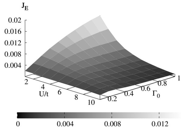
**Figure 5** Energy flow Eq. (12) through a 129-site nanowire as a function of the coupling constant  $\Gamma_0$  and the impurity potential  $U$ . The temperatures of the electrodes are  $k_B T_L = 0.11t$  and  $k_B T_R = 0.01t$ . The bias voltage in the system is zero. The energy flow is expressed in  $(t^2/\hbar)$  units.
