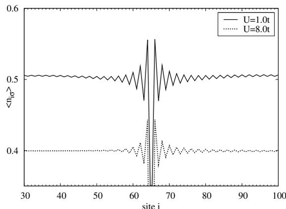
**Figure 2** Occupation of sites in the vicinity of the impurity for a 129-site nanowire. The temperatures of the electrodes are  $k_B T_L = 0.11t$  and  $k_B T_R = 0.01t$ . The values of the impurity potential are indicated in the legend. We have assumed  $\Gamma_0 = 0.5$  and the zero bias voltage. The curve for the  $U = 8.0t$  has been shifted downward by 0.1.
