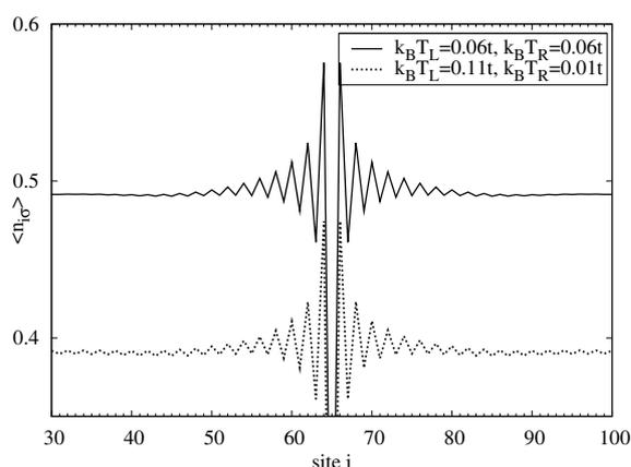
**Figure 1** Occupation of sites in the vicinity of the impurity for a 129-site nanowire. The temperatures of the electrodes are indicated in the legend. We have assumed the impurity potential  $U = 2t$ , the zero bias voltage and the coupling between the nanowire and the electrodes  $\Gamma_0 = 0.1$ . For the sake of the clarity the curve for the  $k_B T_L = 0.11t$  and  $k_B T_R = 0.01t$  has been shifted downward by 0.1.
