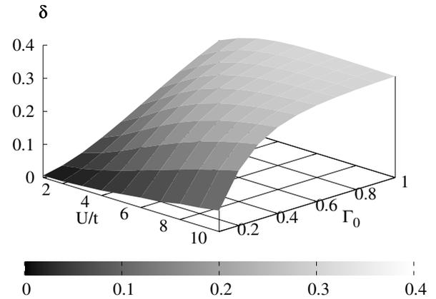
**Figure 4** The asymmetry of the occupation of sites (Eq. 12) for a 129-site nanowire as a function of the coupling constant  $\Gamma_0$  and the impurity potential  $U$ . The temperatures of the electrodes are  $k_B T_L = 0.11t$  and  $k_B T_R = 0.01t$ . The bias voltage in the system is zero.
