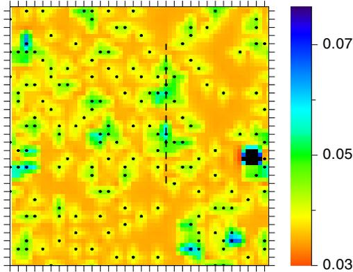
FIG. 3 (color online).  $\Delta_i/t$  calculated for  $U = 8t$ ,  $V_0 = 5t$ ,  $\lambda = 2a$  and  $\bar{n} \approx 0.83$ . The positions of impurities are marked by dots. The dashed line shows the cross section, along which the LDOS presented in Fig. 4 was calculated.
