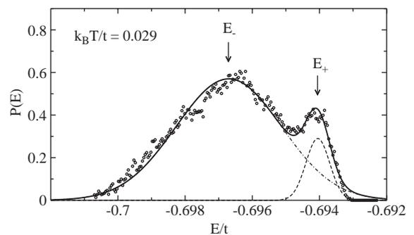
Fig. 1. Probability distribution of the electronic free energy at temperatures close to the critical temperature for  $U/t = 0.5$ . The thick solid lines represent a superposition of two Gaussians that fit the simulation results, whereas the dashed and dashed-dotted lines show the component Gaussians. The arrows indicate positions of the centers of the Gaussians representing low-temperature ( $E_-$ ), and high-temperature ( $E_+$ ) phases, respectively.
